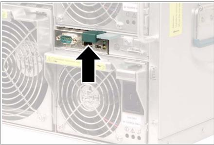
Figure 62: Disengaging the management blade
